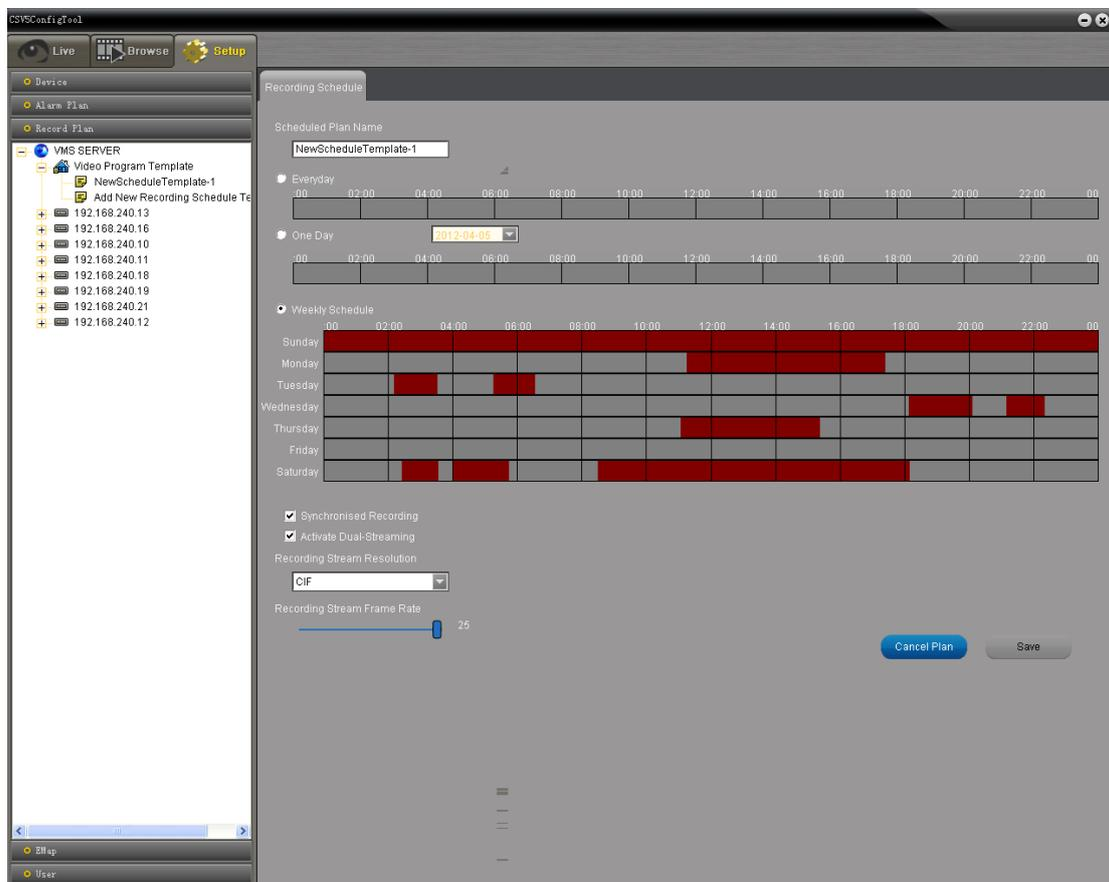
Video plans is to set up each camera as an unit, configure each camera for recording, so the user can design different recording plan according to different camera's angle. It can most effectively use the resource. System administrators will set the video plan
