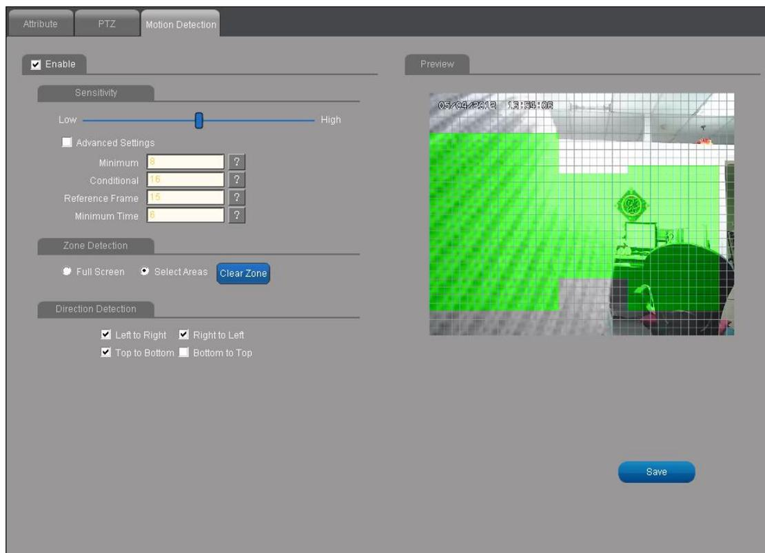
Platform software can achieve dividing a monitoring window into small ones, the user can select random area for detecting area, and set the sensitivity in this detect area. Hence when there is a moving object inside the view, the alarm will be triggered.
