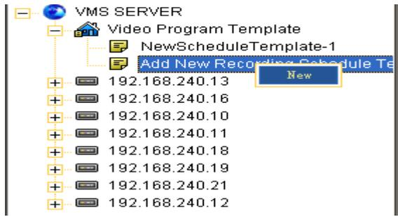
Add a new video plan template to server, in order to facilitate a large number of similar cameras device to directly apply the template parameters of the video program, direct reuse.
