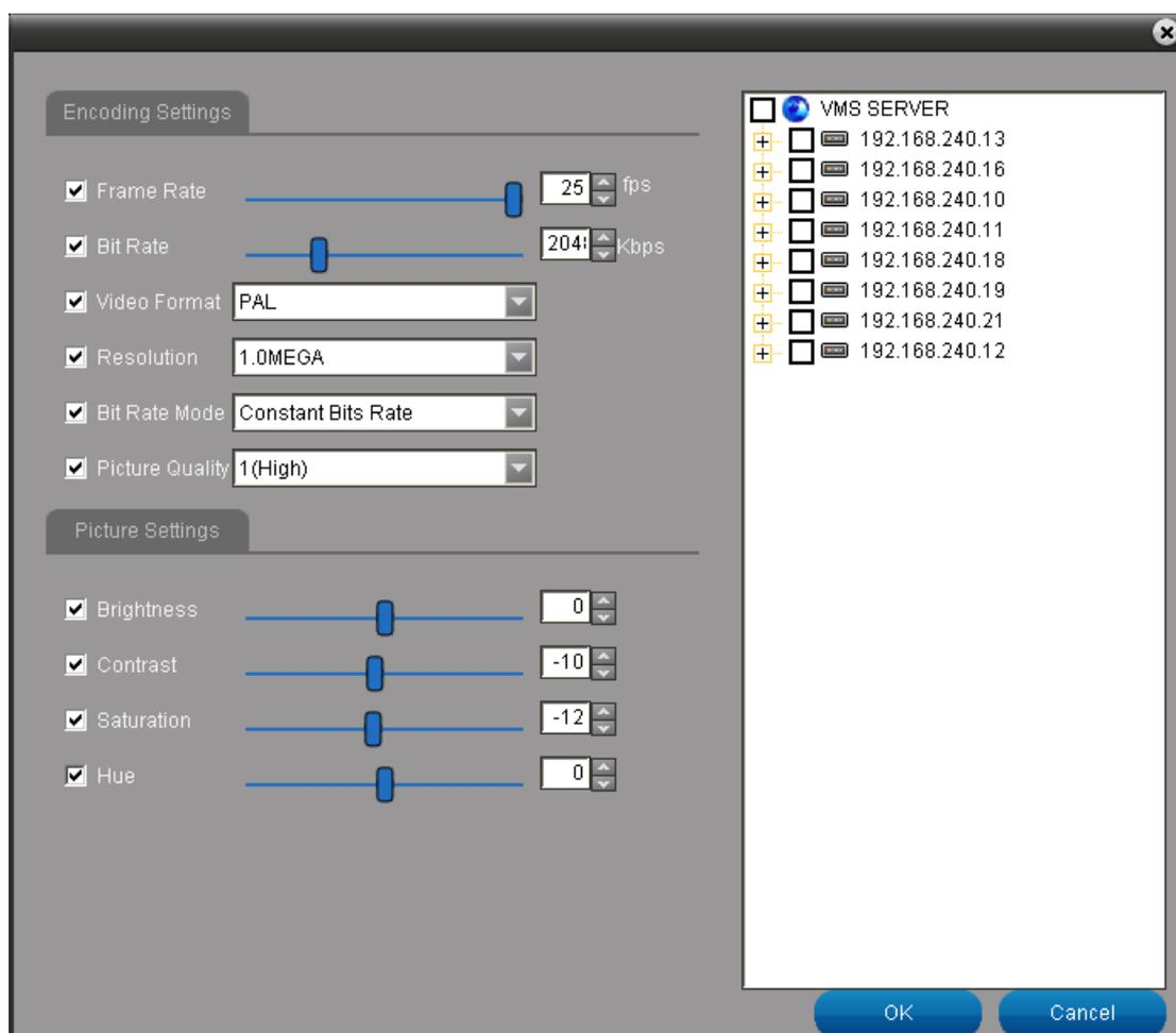
Select the current Video and cameras parameters as a template, other devices in the server list as objects, copy the template camera parameters to other devices in the server.
